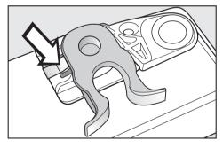
Using a screwdriver, remove spring clamp (1) from underneath the door and fit it on the opposite side.
